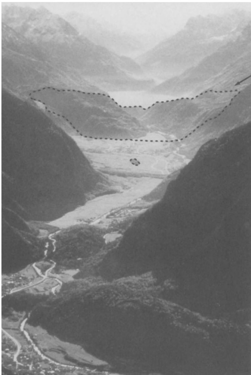
Fig. 2.15. Köfels rockslide. General view from the north. Dotted lines show periphery of deposits with the plateau of Köfels at right, the Maurach gorge in the centre, the Tauerberg at left, and, in front of the gorge's mouth, the separate debris of "Lärchbühl" (connection with Köfels slide uncertain). Arrow indicates direction of displacement (by courtesy of E. Preuss)
