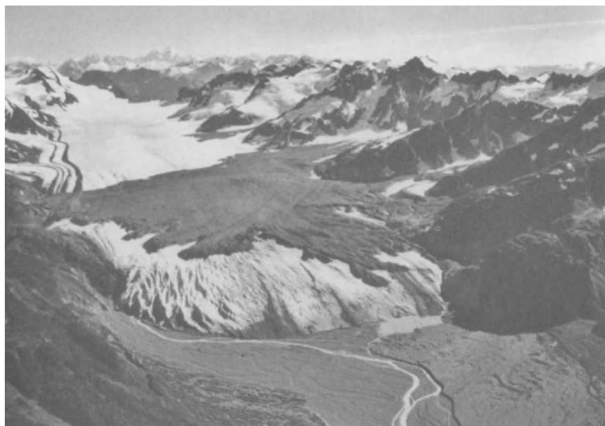
Fig. 2.11. Sherman rockslide of 1964, aerial view from west. The mass originated from the highest mountain visible behind the debris at right (as it lost its top in the event, it is now called Shattered Peak). Note the large extension of the deposits on the glacier (area of ice covered by debris is about 5 km 2 ) and the slight run-up at the extreme left (by courtesy of US Geological Survey, University of Puget Sound, represented by S. M. Hodge)
