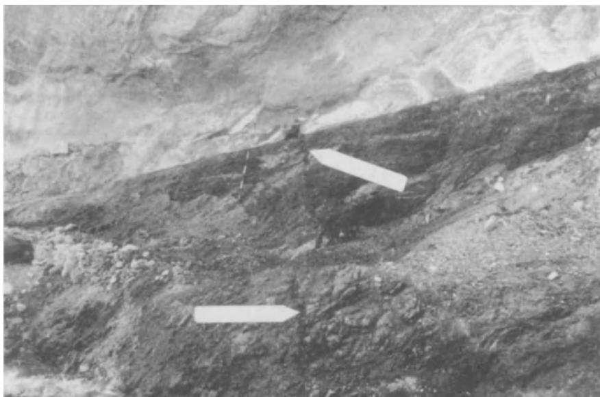
Fig. 2.25. Langtang rockslide. Main sliding surface with layer of glassy, predominantly compact frictionite. Arrows show transverse crack filled with frictionite even at a considerable distance from the sliding surface. Note the almost perfect straightness of the surface. Division of stick is 0.1 m (by courtesy of H. Heuberger)
