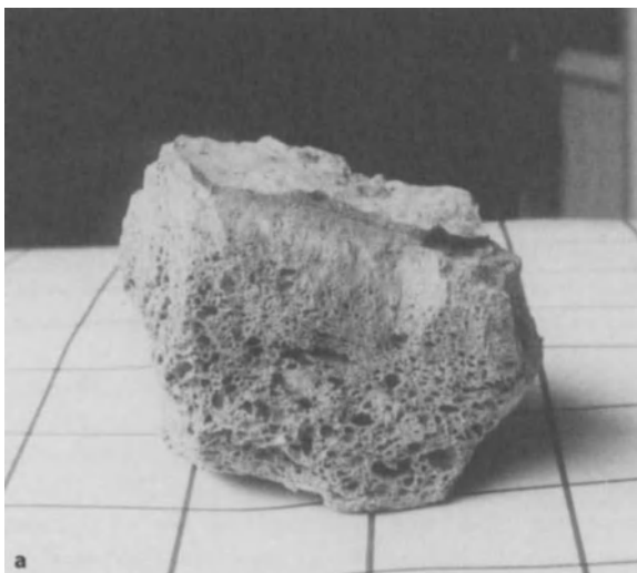
Fig. 2.19. Köfels rockslide. Fused rocks (frictionites). a typical porous, pumice-like piece (squares are 50 mm); b section through specimen showing low viscosity of melt (thickness of gap is about 10 mm) (by courtesy of E. Preuss)
