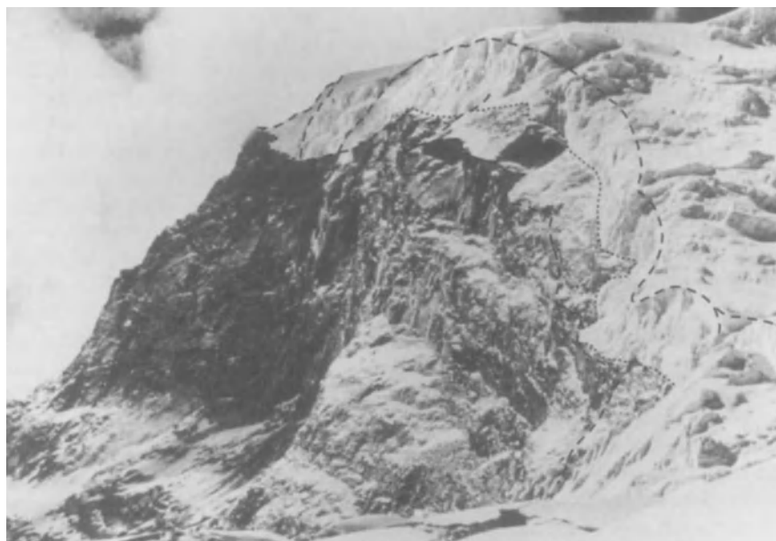
Fig. 2.49. Huascarán event, headscar and steep wall. Broken line shows approximately the periphery of the displaced material. The photo, taken soon after the event, clearly illustrates the difficulties encountered in estimating the initial volume of the mass (by courtesy of W. Welsch)
