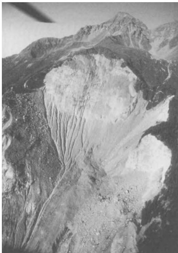
► Fig. 2.29. Val Pola rockslide, aerial view of scar with Monte Zandila in the background. Photo taken few days after event. Note characteristic details: channeling geometry of lateral surfaces, particularly well-developed on the left; beginning erosion by two torrents; the one at right is Pola (photo by unknown helicopter pilot having taken part in rescue; by courtesy of the former Swiss Federal Office for Military Airfields)
