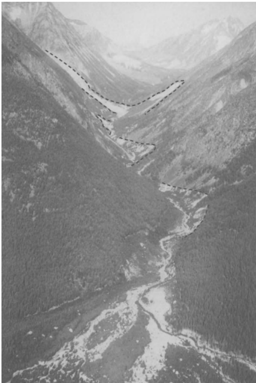
Fig. 2.3. Pandemonium Creek rockslide, “bobsleigh run” through Pandemonium Creek Valley, view from east. Dotted lines , background: traces of motion in descending (left) and running up (right). Dotted lines in valley: marks of superelevation used as “speedometers”. Foreground: first half-kilometre of run-out area (by courtesy of the Geological Survey of Canada, Ottawa, Ontario, represented by S. G. Evans)
